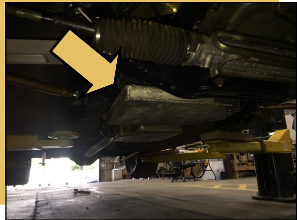
The modified oil pan sitting above the subframe.
