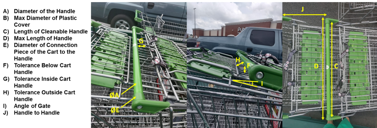
Fig. 26. Clearance Measurements for UV-C Delivery Device Optimization.
